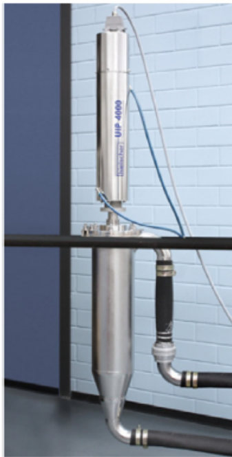
Fig. 11. Industrial ultrasonic continuous equipments (Hielscher - www.hielscher.com ).
