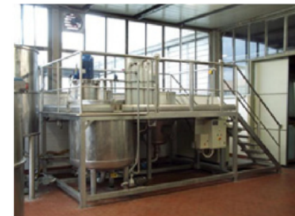
Fig. 12. Industrial ultrasonic batch equipments: 50, 500 and 1000 L (Reus - www.etsreus.com ).
