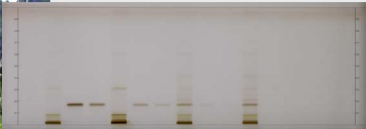
HPTLC chromatogram for determination of catalpol. Four samples of Plantago lanceolata (track 1, 4, 7, 10) and nine catalpol standards (track 2, 3, 5, 6, 8, 9, 11-13)
