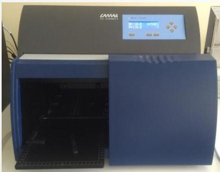
scanner, CAMAG TLC scanner 4
